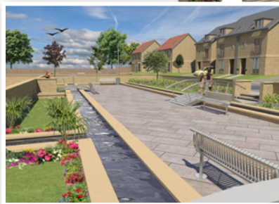
Marshalls linear drainage into open drainage canal
