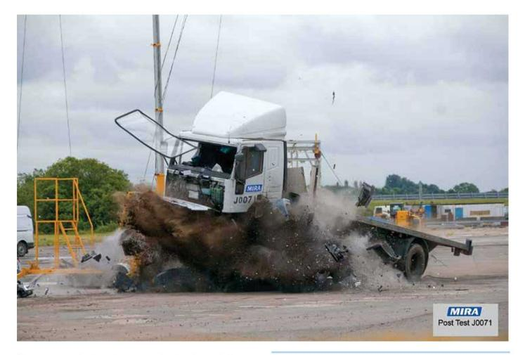
The testing methods and criteria outlined in the workshop agreement are a combination of those outlined in the BSI PAS 68, 69, CEN and American ASTM standards. As such, any products that have been successfully tested to the requirements of IWA are also approved to the requirements of all previous standards as well (PAS68, PAS69, CEN, International American Standards).
