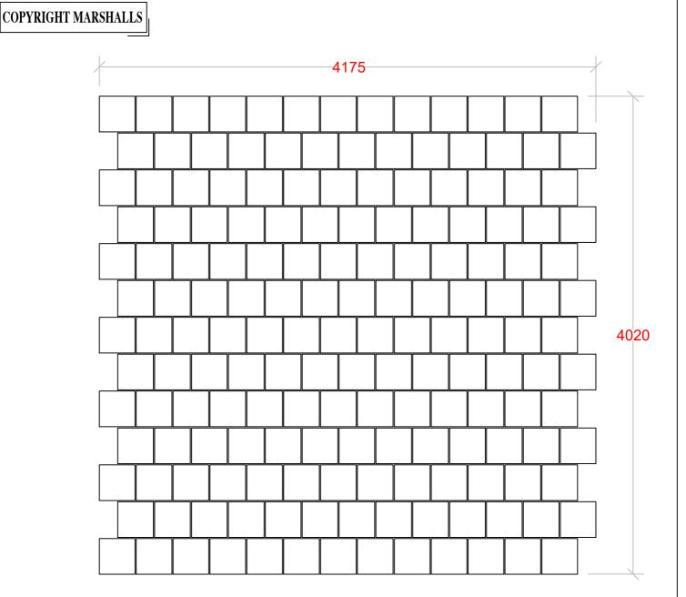
Stretcher Bond (Mortar bed and 10mm nominal mortar joint required)
