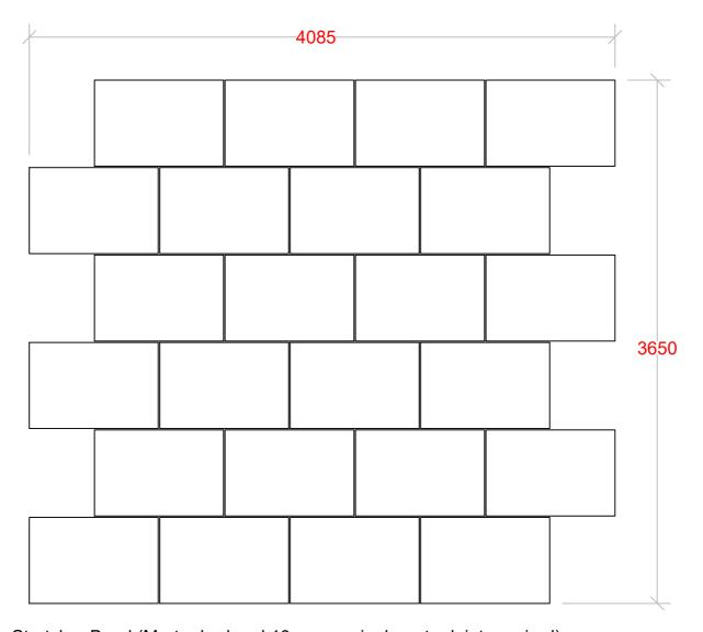
Stretcher Bond (Mortar bed and 10mm nominal mortar joint required)
