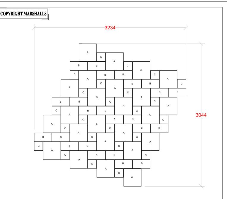
Repeatable Random Pattern (Mortar bed and 10mm nominal mortar joint required)
