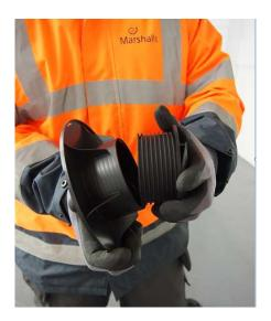
For best results, ensure you use the rubber base pads on the sub-base to keep the pedestals in place and rubber head pads on the head of the pedestal to reduce noise and minimise movement of the paving units. If laying vitrified paving onto a roof terrace or where wind loading may be a concern, apply a small dab of Sika EBT onto both sides of the rubber head pads before installing the paving unit to minimise movement.
