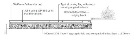
Typical section through a patio constructed in accordance with Marshalls Register Installation Procedures
