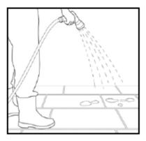
Thoroughly saturate the paving surface. It is impossible to over water the paved area. Failure to wet the paving correctly could result in temporary staining of the paving surface.
