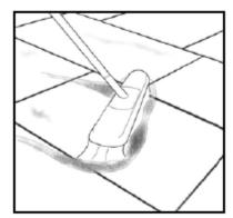
Sweep off any excess jointing compound and store remainder in the tub. Fill tub to the top with water making sure the entire jointing compound is covered by at least 80mm (3 inches) of water. Product can then be stored for up to one year as long as the product remains fully immersed in water.
