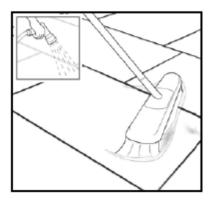
To finish the process, gently spray the surface with a wide angled spray and brush excess joint compound off the surface using a soft bristled brush.
