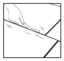
Strike off the joint using a Marshalltown jointer or similar tool. Top up any sagging joints with more jointing material and strike again if required.
