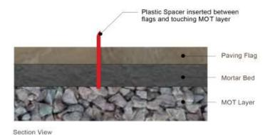
Once the mortar bed has partially cured remove the spacers and introduce Symphony Jointing Compound.
