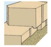
Minimum external and internal radius – 750mm on the bottom course.
