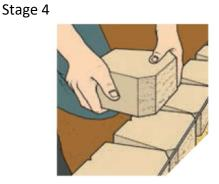
Each course must be backfilled accordingly. The backfill zone consists of 300mm of free draining material followed by backfill material. The backfill zone should be at least equal to the wall height.
