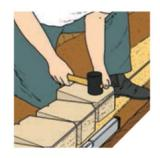
Position the first course of blocks side by side to required line and level the blocks in both directions.
