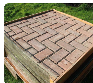
Paving rig with geotextile.
