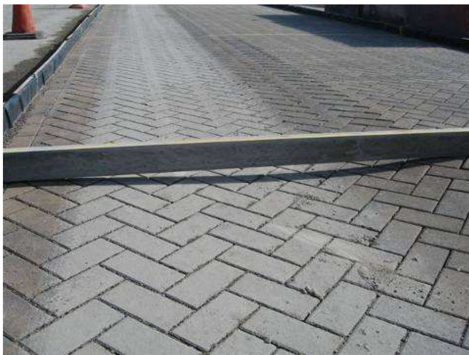
Figure 15. Typical rut in Test Item 1 after several thousand standard axles.
