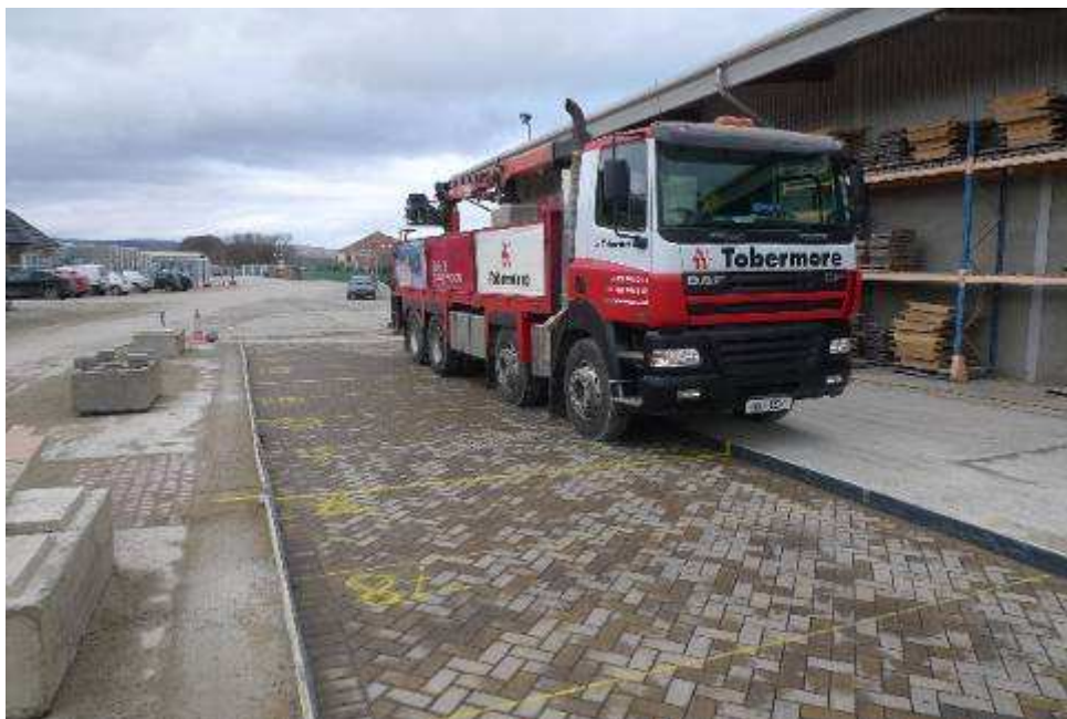
Figure 14. Trafficking was by means of an overloaded eight wheel truck which shuttled back and forth at a constant speed of approximately 10mph (16kph).
