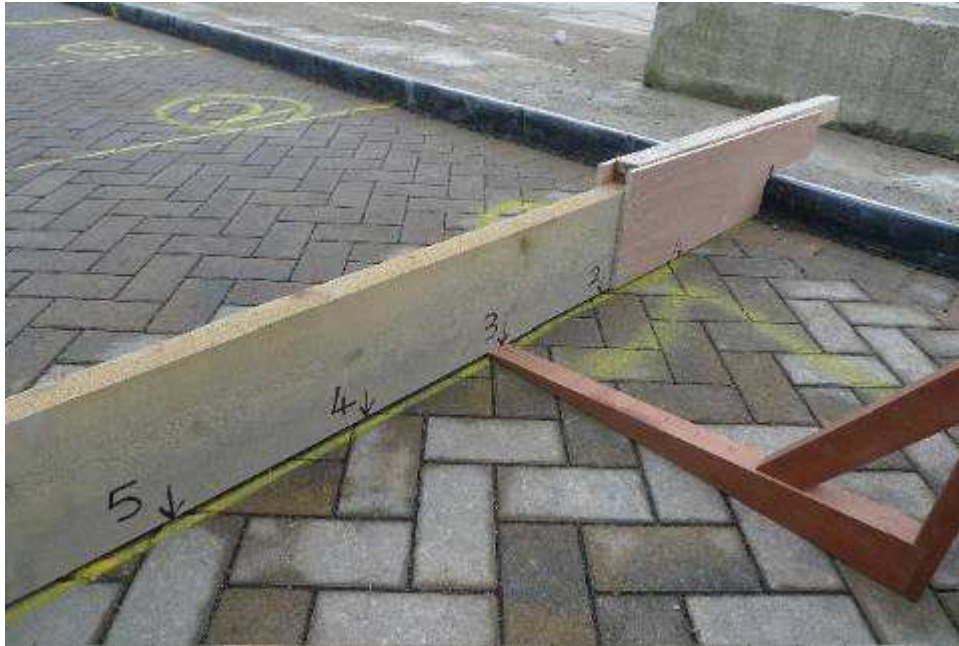
Figure 13. Values of permanent deformation were measured at locations as marked on the board. Each measurement point occupied a similar position in relation to the paver laying pattern. Measurements were taken by inserting the calibrated wedge between the pavement surface and the straight edge. An initial set of readings was taken prior to trafficking and all reported readings are obtained by first subtracting the initial data set.
