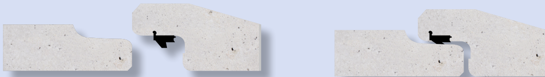
Fig. B2. Integral sealing ring - standard for most UK concrete pipes
