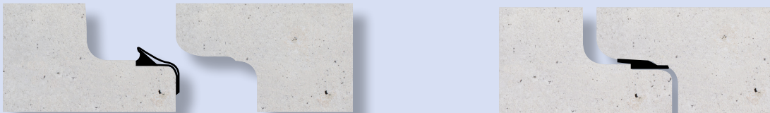
Fig. B3. Pre-lubricated Sliding Ring
