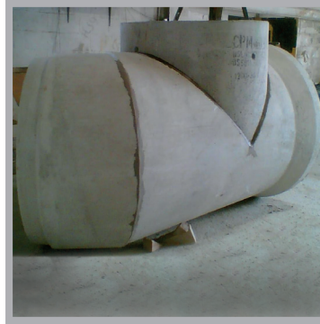
1200mm side entry being manufactured
