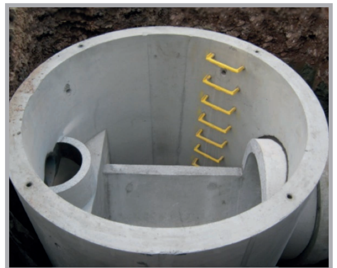
2100mm diameter wide wall manhole complete with pre-fitted ovoid butt and channel plus internal back-drop junction
