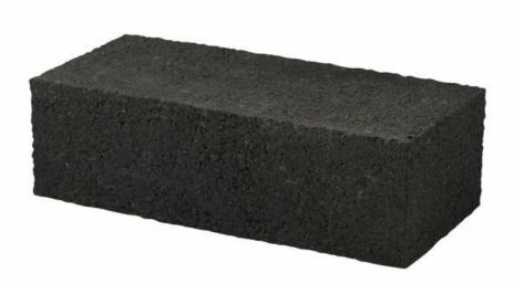
Marshalls **coursing bricks** are designed to be used in all types of construction in conjunction with dense aggregate or lightweight aggregate blocks, both of which are available in standard bed widths of 100mm and 140mm. "They are also available as 40mm high slips for use in building up courses in beam and block floors".
