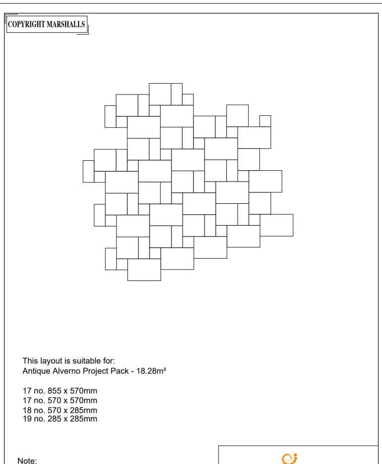
All dimensions, and coverage rates, are those attained when laid with a 10mm joint. An additional allowance is normally required for cutting purposes depending on the complexity of the pattern and overall layout of the area.
