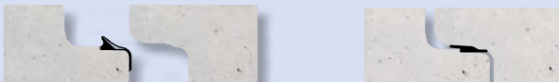
Fig. B3. Pre-lubricated Sliding Ring
