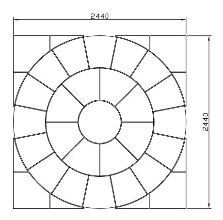
Circle Pattern (Mortar bed and 10mm nominal mortar joint required) Suggested layout using:
