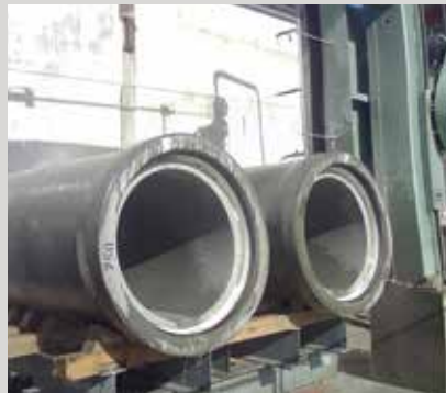
Marshall's has invested in the only 'rope' saw of its kind currently working in the UK, which can cut multiple pipes
