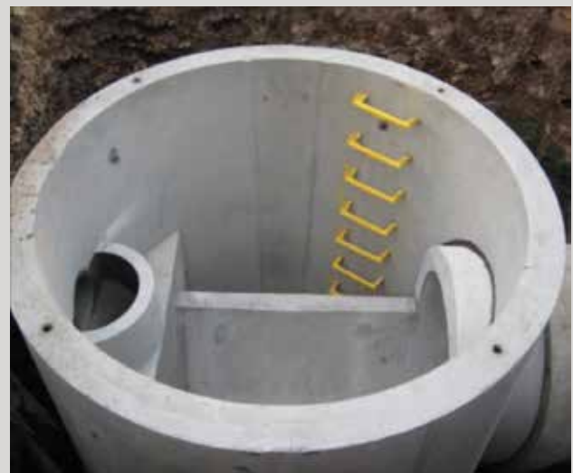
2100mm diameter wide wall manhole complete with pre-fitted ovoid butt and channel plus internal back-drop junction
