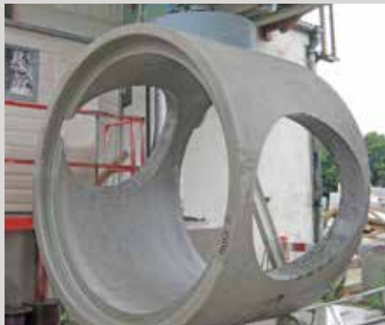
1800mm sealed manhole being cored for a 900mm internal diameter pipe
