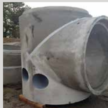
1600mm off 1600mm flow control chamber
