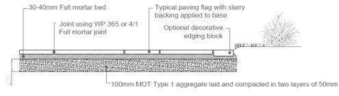
Typical section through a patio constructed in accordance with Marshalls Register Installation Procedures
