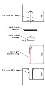
• The sealing material can then be laid around the sections joint circumference, taking care to carefully pierce the locating dowels through the material so that it lies flat against the spacing washers. The purpose of the washers is to maintain a minimum 5mm joint gap for the sealing material between the two jointed surfaces when under compression.
