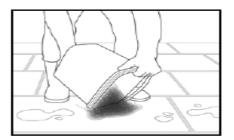
3. Brush the material in to the joint diagonally (at a 45° angle). Ensure that the joint void is completely filled. See the Illustration below. The jointing material should be used within one hour of pouring the vacuum pack.
