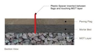
Once the mortar bed has partially cured remove the spacers and introduce Symphony® Jointing Compound.
