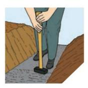
Dig a trench to the depth of a full block plus 150mm for foundation material. The width should be minimum of 2 times the wall thickness and the foundation material should extend 85mm to the front and rear of first course block.
