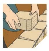
Each course must be backfilled accordingly. The backfill zone consists of 300mm of free draining material followed by backfill material. The backfill zone should be at least equal to the wall height.
