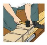
Position the first course of blocks side by side to required line and level the blocks in both directions.
