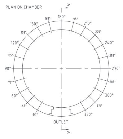
Please note that there is a 1 in 9 gradient for the 1200mm perfect manhole and a 1 in 18 gradient for pipes 450mm upwards for the 1500mm perfect manhole and the angles between adjacent connection cannot be less than 24 degrees.
